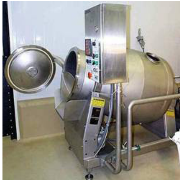
Above is a meat tumbler machine. This can be used to distribute the marinade solution in the meat.
